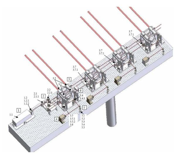
Figure 1 Layout and identification of components on the metrology bench.
