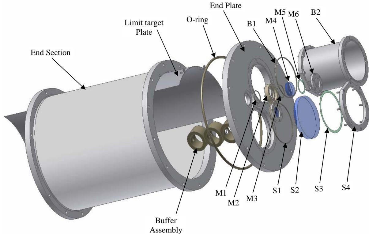
**Figure 4 BCA End Plate.** Components marked with a number prefixed by M are metrology window components, those prefixed by S are science window components and those prefixed by B are beam relay interface components. See text for a descriptive key to these components.
