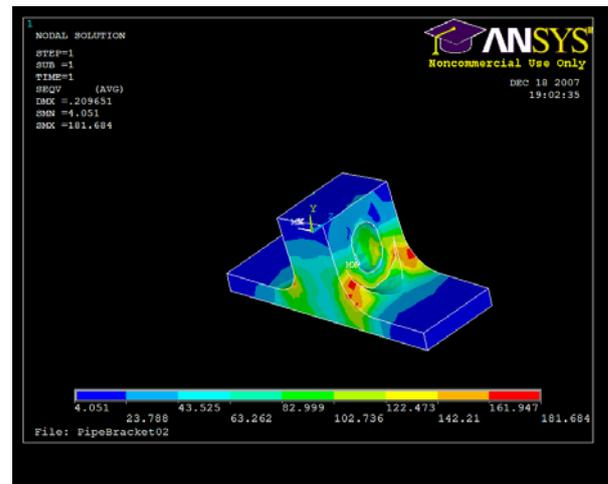
Figure 29: Von Mises stress for pipe bracket
