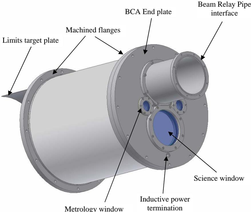
Figure 2 The BCA end section with the end plate carrying the metrology windows, the science window and the connection to the beam relay pipe. The end of the limits target plate is just visible at the left hand side.
