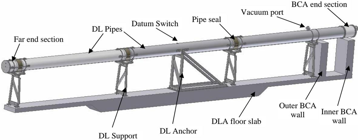
**Figure 1 A 3-D view of the delay line nearest to the BCA. The wall between the DLA and the outer BCA and the wall of the inner BCA are shown. The anchor and the supports either side are positioned over the thickened floor slab. The end of the pipe at the left shows the end section that would be at the far end of the delay line. The locations of the datum switch and the vacuum port are also shown**
