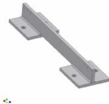
**Figure 15 Delay line support base plate.**
