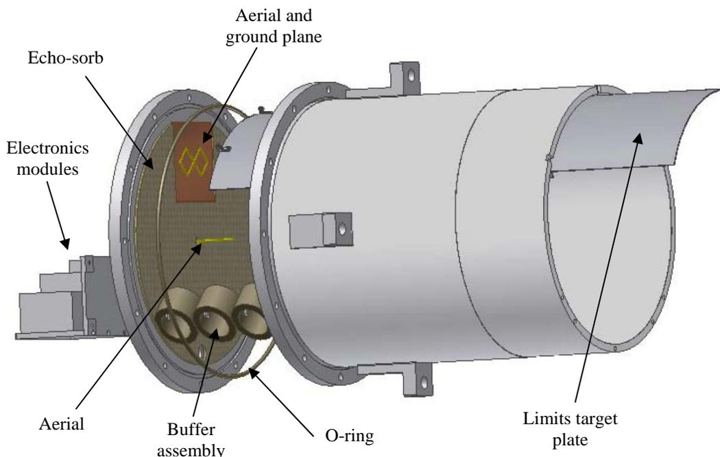
**Figure 7 Exploded view of the Far End Plate showing the buffer assembly, the O-ring seal, the aerials, the ground plane and the echo-sorb arrangement.**
