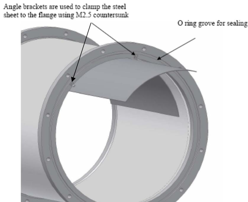
Figure 6: End section with target plate fitted.
