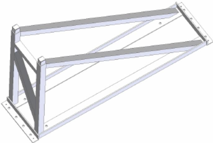
Figure 20: The anchor frame
