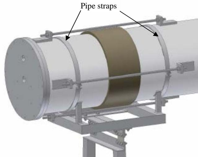
**Figure 14: A pipe joint showing the cradle and the straps holding the pipe to it.**
