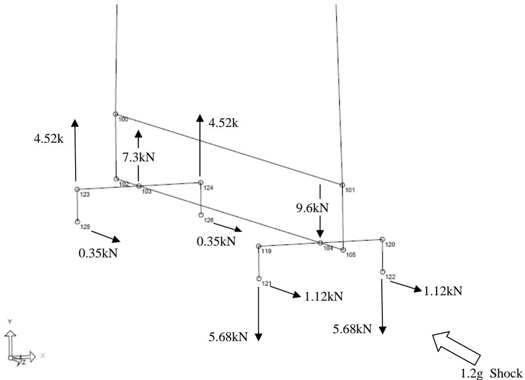
Figure 23: Maximum force at ground connection points and in members of support 4 due to a 1.2g lateral shock. Note: for axial loads compression is -ve.
