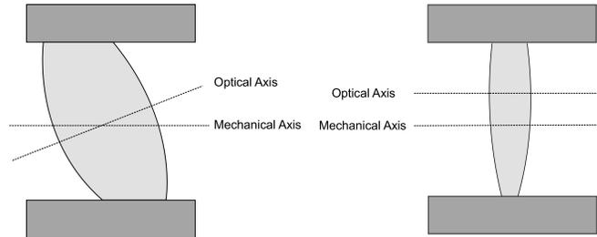
Figure 2: Lenses suffering from errors in tilt (left) and centration (right). The former is characterised by the angle between the mechanical and optical axes. The centration error is quantified by the distance between the two axes perpendicular to the direction of beam propagation.
