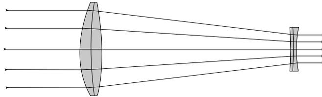
Figure 1: A schematic diagram of the beam compressor to be used immediately in front of the Agilent laser head. The collimated beam from the head enters from left and is compressed before exiting the system, still collimated, to the right.
