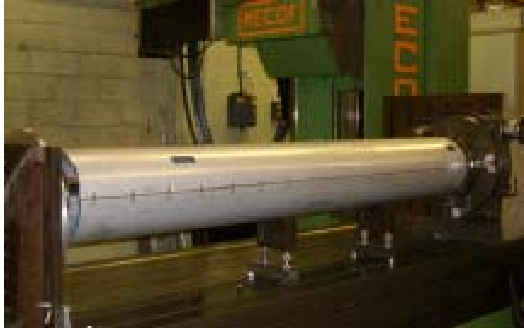
Figure 6: A photograph of the trolley shell during manufacture showing one of the longitudinal joints. The holes for the wheels have just been machined.
