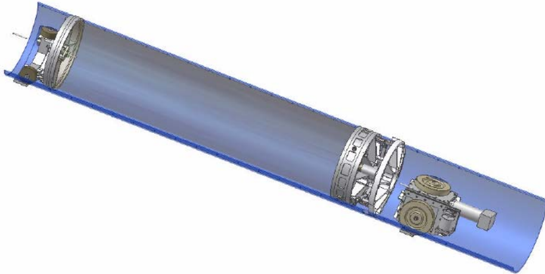
Figure 9: A 3-D view of the trolley design showing the components that need to be aligned to the trolley axis. These are: the front wheel assembly, the front cat's eye wishbone leg, the rear cat's eye wishbone leg, the voice-coil bulkhead and the rear wheel drive and steering assembly.
