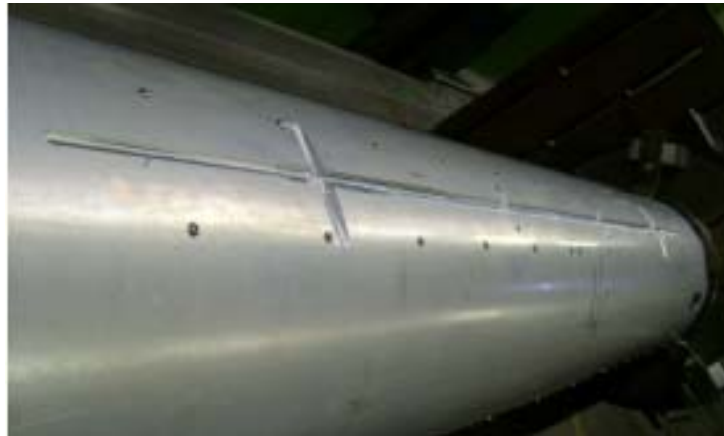
Figure 7: A photograph of the underside of the trolley chassis showing the slot for the inductive power transformer. The transverse slots are for transformer supports and electrical connections. The small holes are the fixing screw locations for the glued segments.
