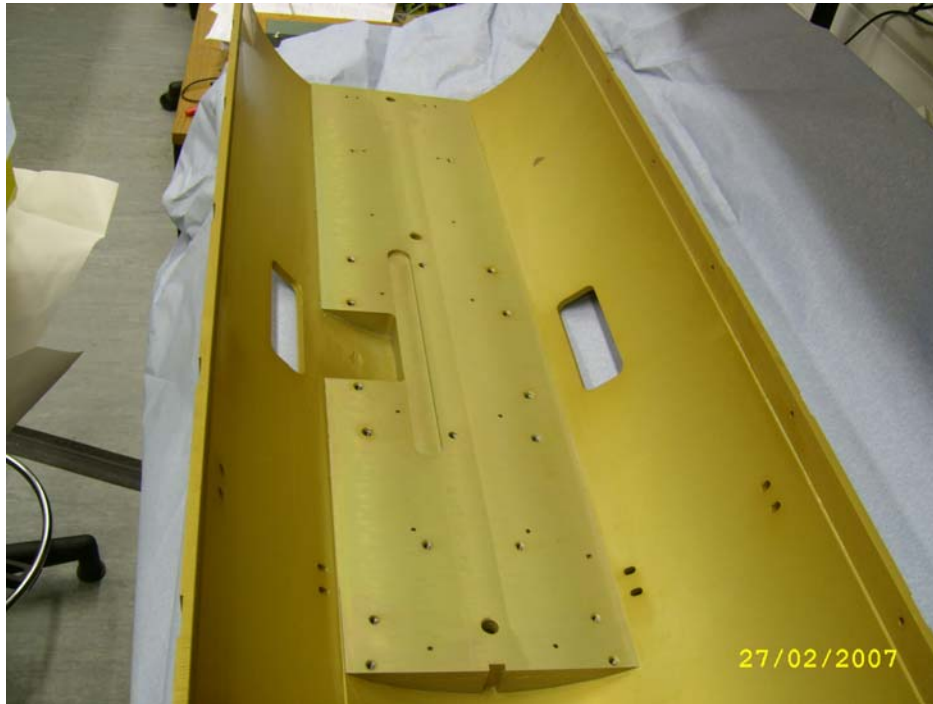
Figure 25: Carriage chassis with rear segment fitted.
