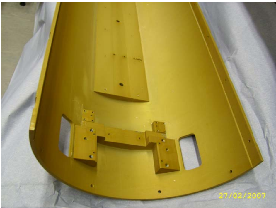
Figure 26: Carriage chassis with intermediate and front segments fitted.
