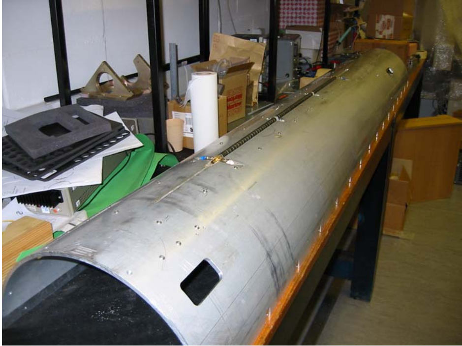
Figure 29: Inverted view of chassis with inductive power transformer in situ.
