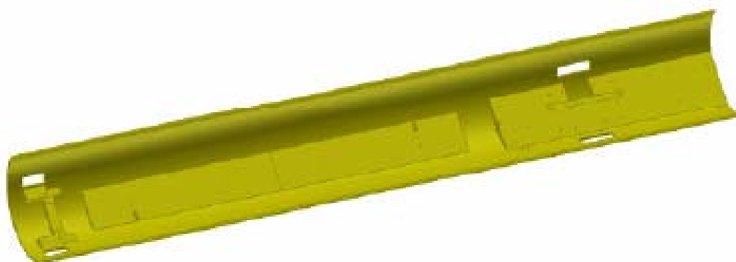
Figure 8: The trolley chassis showing the holes machined for the wheels and the four segments forming the machined base to which the trolley components are fixed.
