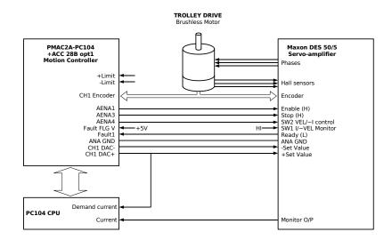
Figure 2: PMAC arrangement for control of the trolley drive.
