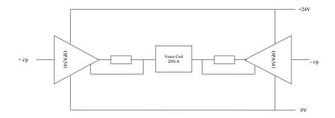
Figure 5: Voice coil power amplifier schematic.
