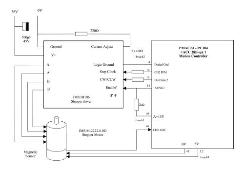
Figure 3: PMAC arrangement for control of the steering motor.
