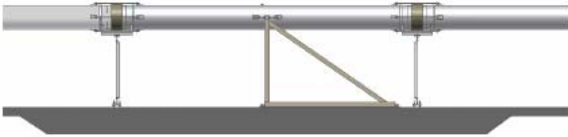
**Figure 6** The anchor is positioned between two supports.
