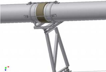
**Figure 9:** Completed pipe joint with seal and draw bars in position and the pipe clamped to the cradle.
