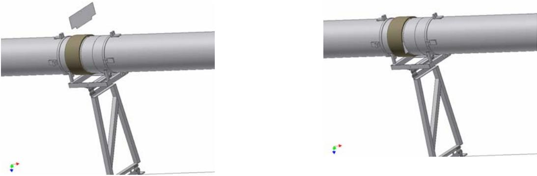
**Figure 8:** Installation of a pipe onto a stand showing the seal displaced to allow the pipe target to be inserted. (The pipe draw bars are not shown).
