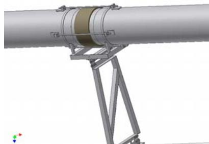
**Figure 9:** Completed pipe joint with seal and draw bars in position and the pipe clamped to the cradle.
