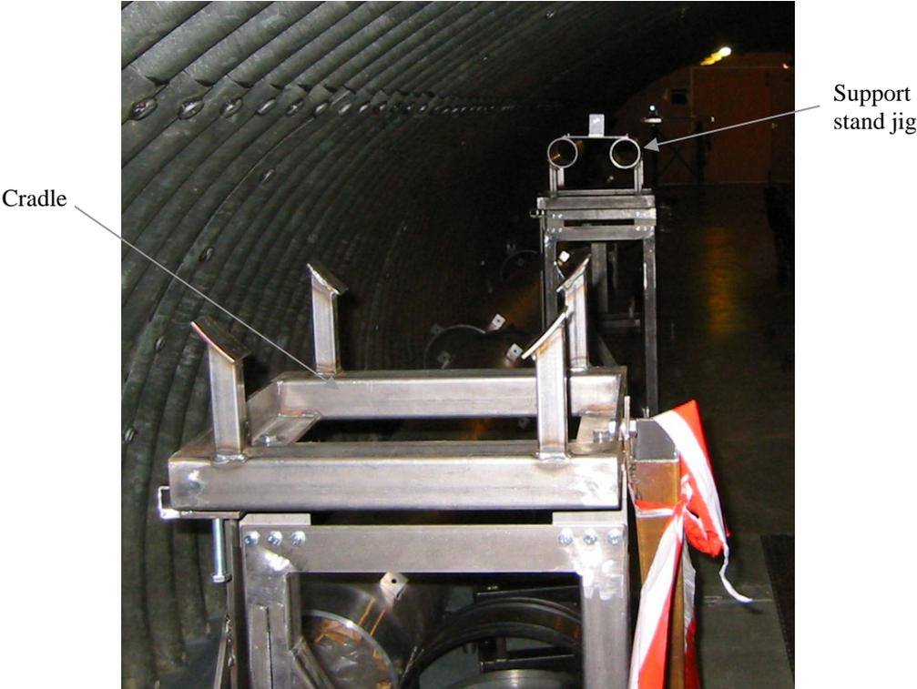
Figure 2: A support stand and cradle is in the foreground and the support stand target is mounted on a stand and cradle in the background
