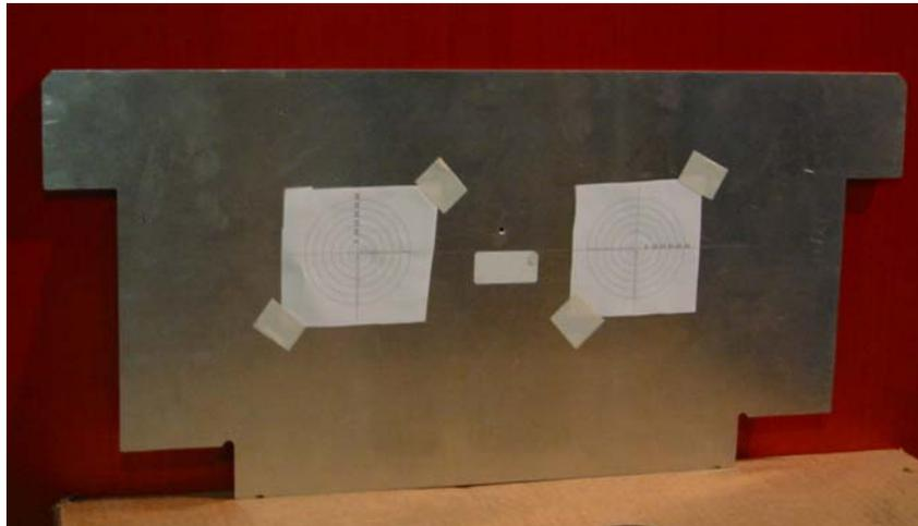
**Figure 5 Photograph of the pipe target used to erect the delay line test rig at COAST. Additional paper targets were added to assist in alignment of the laser metrology system.**
