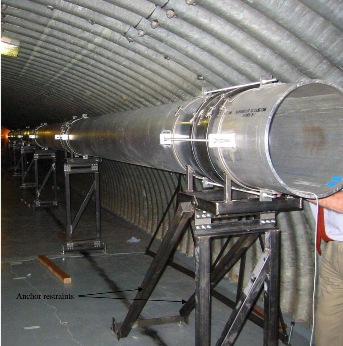
Figure 10: Test rig installed at COAST showing the anchor struts being used to stabilize the nearest support.
