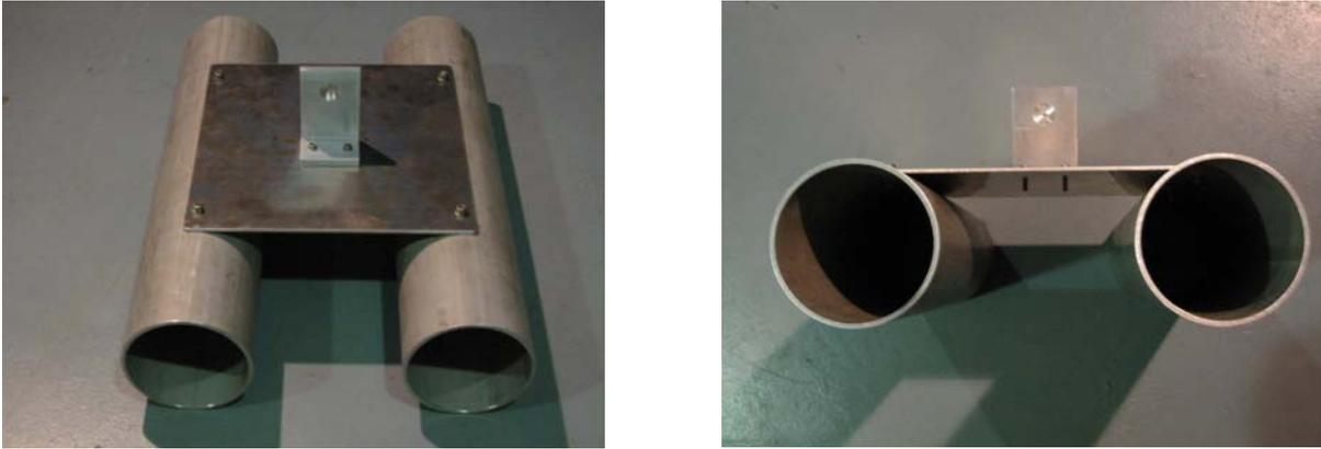
Figure 1: Two views of the support stand alignment jig. The separation of the two pipes places the pin-hole target on the pipe axis when the jig is supported on the cradle tabs.
