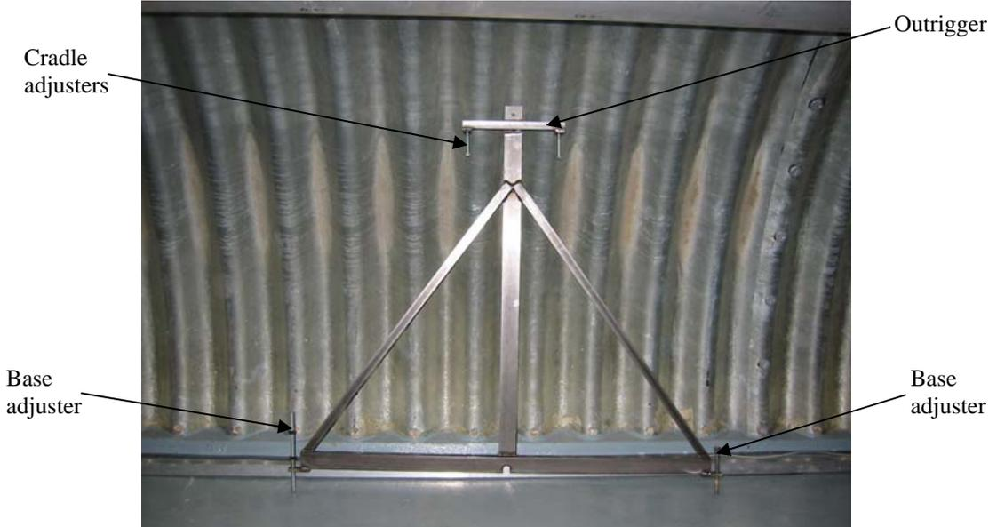
Figure 3: The support stand jig used to stabilize the stand during assembly of the delay line test rig.
