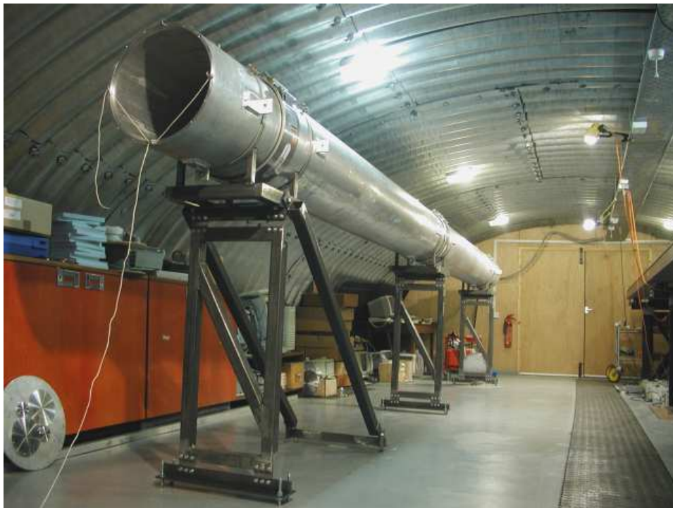
Figure 3.3: Photo of the test rig from the north end showing the longitudinal restraint (behind the northernmost flexure).
