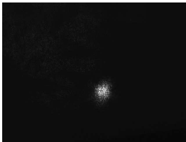
Figure 4.3: An example of a laser spot imaged by the camera. The “graininess” in the image is due to laser speckle.
