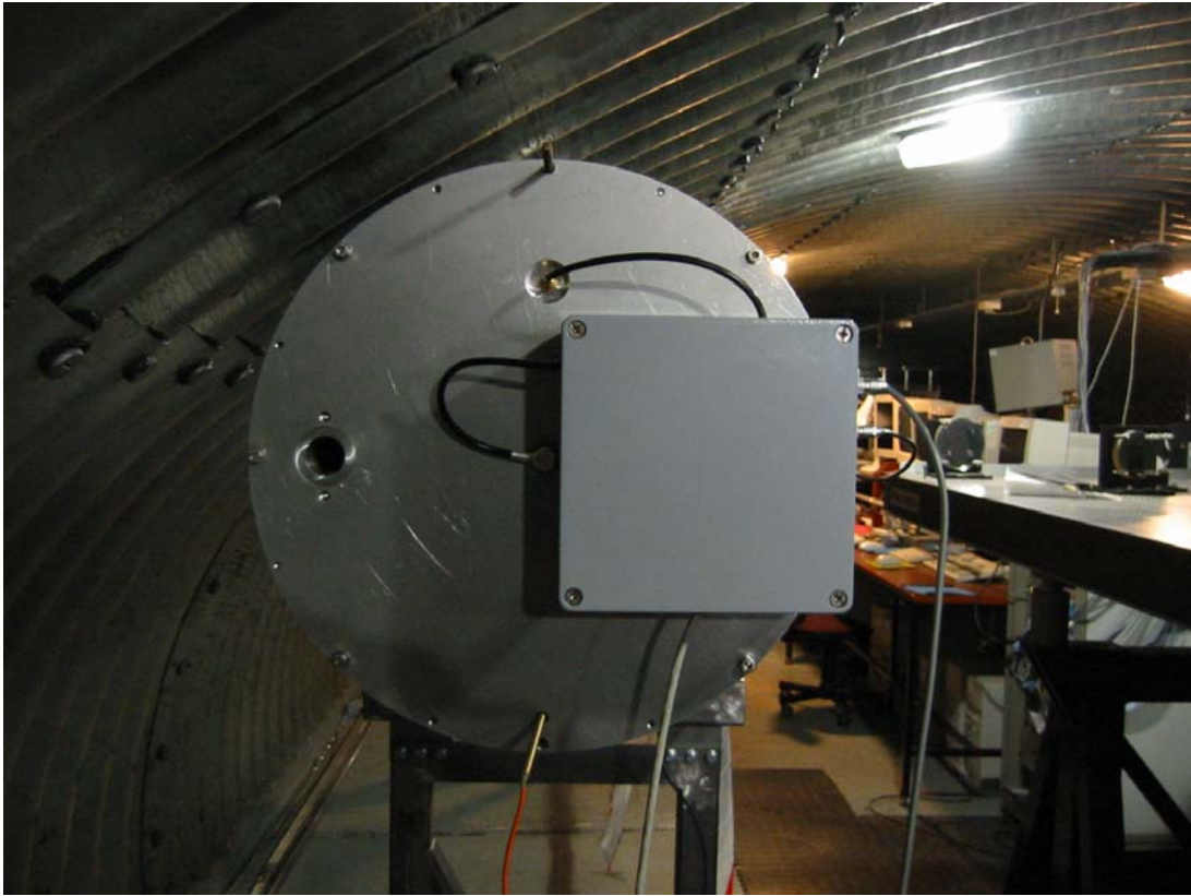
Figure 6 The end plate of the test rig carries the communications module, as at MROI, but not the inductive power module. The inductive power cable termination is at the bottom of the end plate and a vacuum pumping port is on the left. The low-latency link connects at the centre of the end plate and the wi-fi link connects above it.
