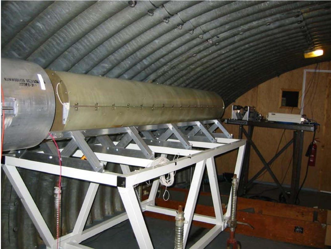
Figure 4 Production trolley on the gurney and about to be loaded into test rig.
