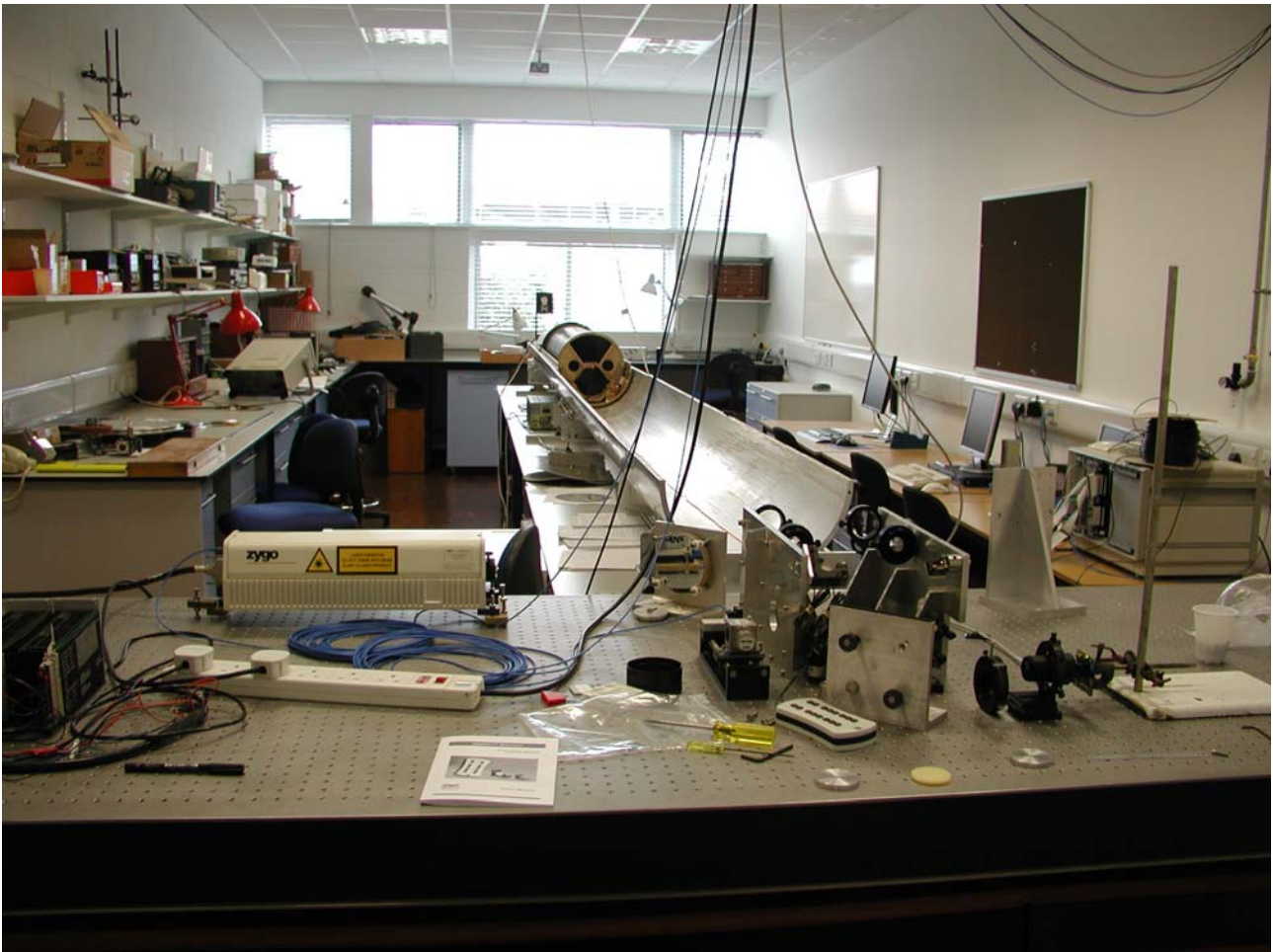
Figure 2: The trolley in the test track with the laser metrology system in the foreground
