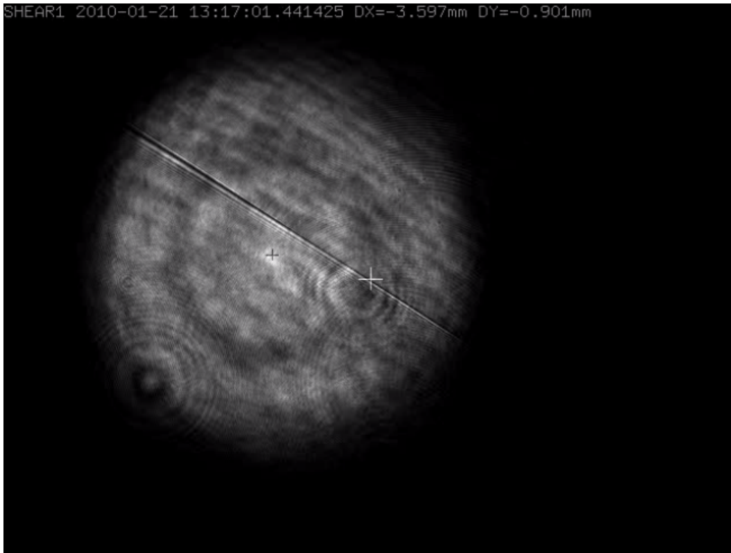
Figure 3: Frame of logged video from the shear sensor program, showing the annotations. The large crosshair is the fiducial point, the small one is the calculated centroid. The diagonal line across the image is an artifact of the beam reducer and does not significantly affect the centroid calculation. In this case the servo is off so that the crosshairs are deliberately separated.
