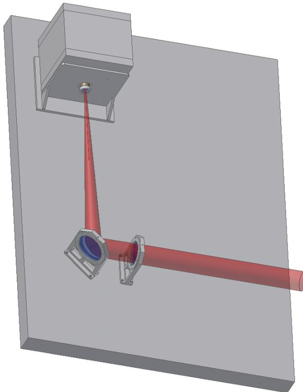
The folding mirror mount has a somewhat higher requirement on stability than the lens mount and will be based on the mount design for the FTT/NAS fold mirrors. The mirror will be pre-loaded against an axial reference face by the retaining ring and held radially by two reference surfaces and a compliant pre-load surface (see Figure 3).
