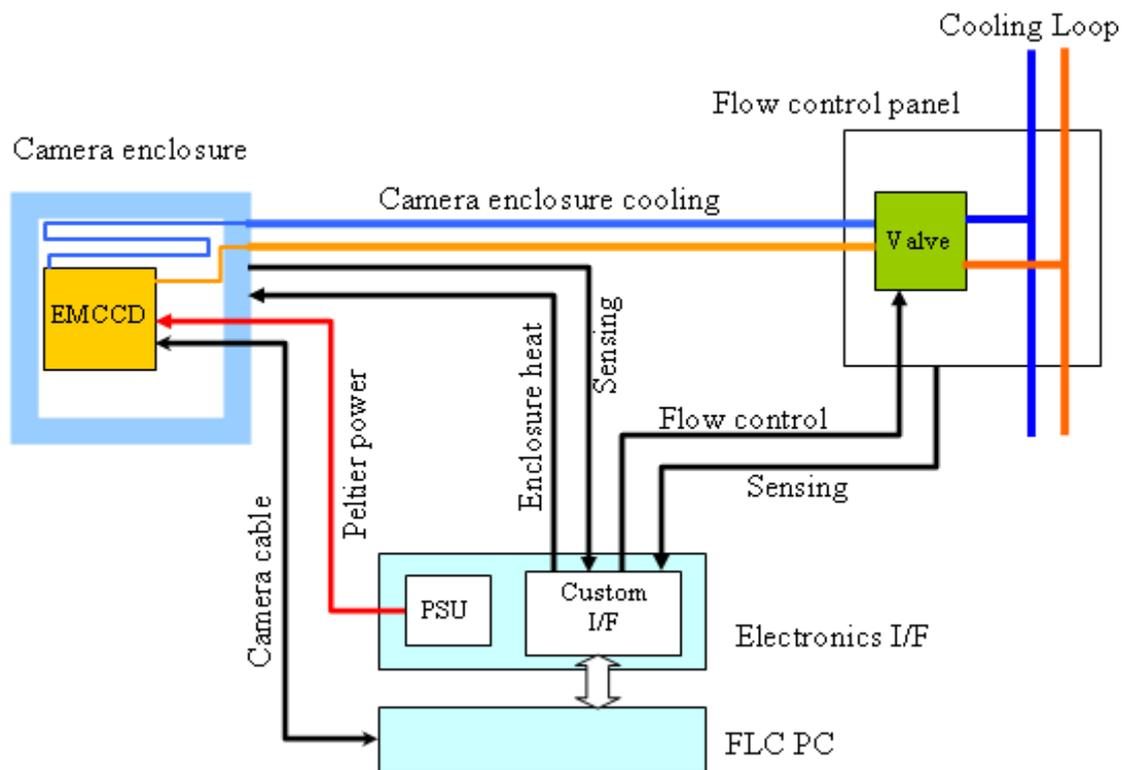
**Baseline design** The preferred approach to cooling of the camera enclosure and the camera itself is to use the EIE electronics housing cooling loop (referred to as Loop 1). Connections to this loop will be brought to an interface at the south edge of the Nasmyth optical table. Here a flow valve, controlled by the FLC computer in the Q5 electronics housing, will provide an appropriate flow through the camera enclosure and camera.
