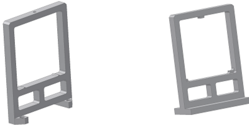
Figure 9: Conceptual designs of the dichroic mount with different clamping methods: (a) mount bearing on the edge of the dichroic, and (b) mount bearing on the face of the dichroic.
