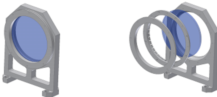
Figure 10: Focus lens and mount. The lens clamping method is designed to maintain the lens centrally in the mount to within 0.4 \mu\text{m} over temperature changes of up to 5^\circ\text{C} . A cemented lens design has been assumed.
