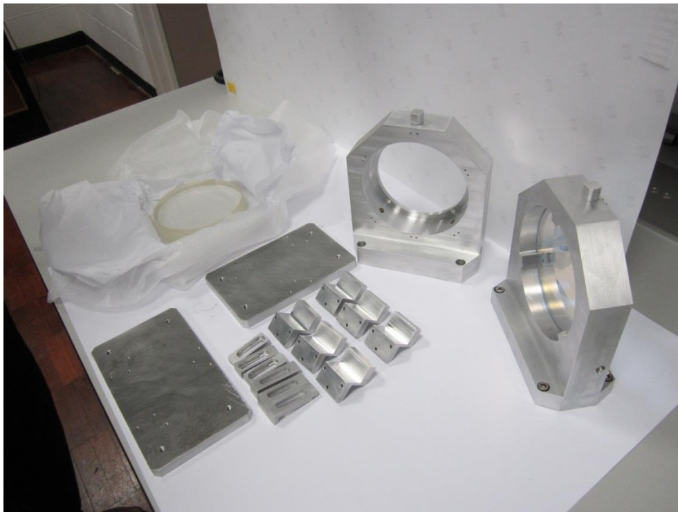
Figure 1: FLC optics and mounts. The two mounts are on the right hand side of this picture and one (to the right) has the optic fitted while the other optic is in the paper wrapping on the left hand side. The base-plates and support legs are in the lower left of the picture together with clamps that will secure the base-plates to an optical table at the telescope. The 2 push blocks, used for adjusting the position of the camera to focus it, are not shown.
