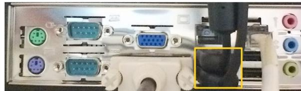
Figure 3: Ensure that any USB devices use the rear USB connectors in the yellow rectangle.
