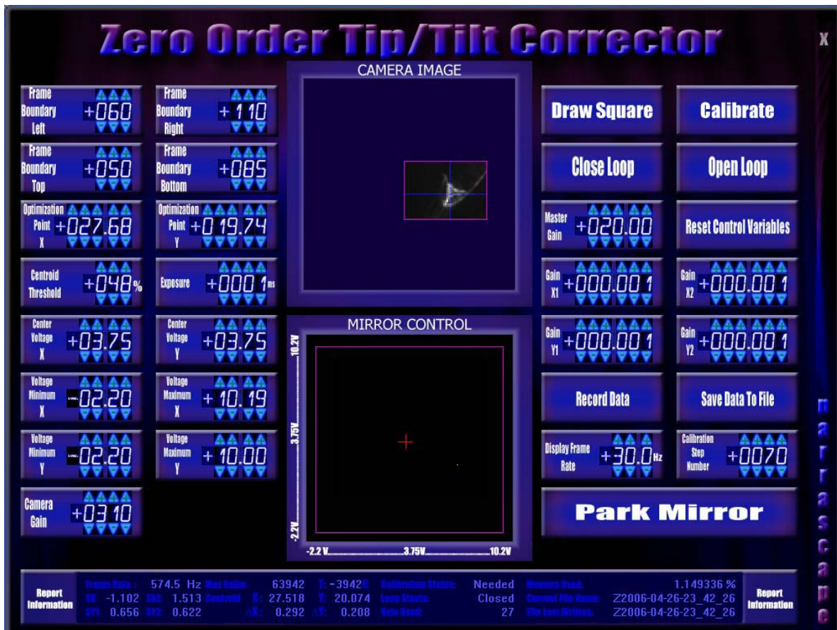
Figure 8-1. Sample GUI with real-time feedback of mirror position, camera image and other telemetry items. GUI also displays control buttons with graphical feedback for control of system parameters.
